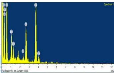
Fig 3: EDX of the formed scale
