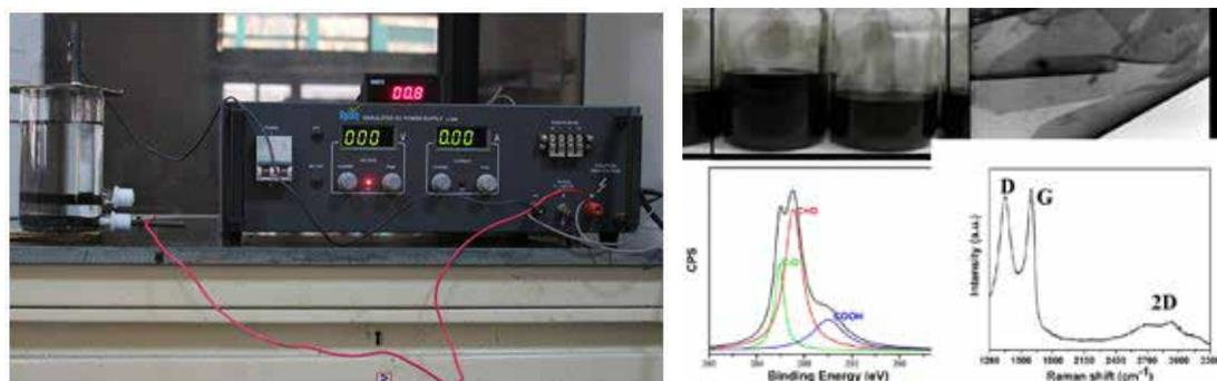
Fig. 1 (a) shows experimental setup, (b) GO dispersed in ethanol solution, (c)TEM image of GO, (d) XPS spectra of GO and (e) Raman spectra of GO.
