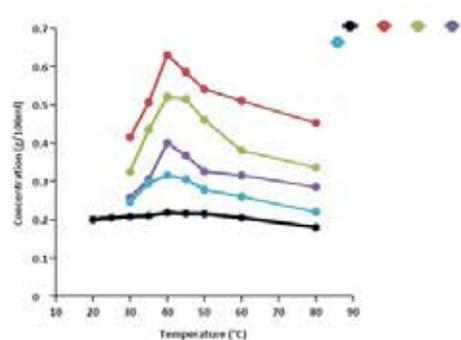
Fig 2: Comparison of solubility's of CaSO<sub>4</sub> in water and in different NaCl- water concentrations
