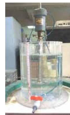
Fig 1. Experimental setup of the stirred tank reactor (6-blade Rushton turbine)
