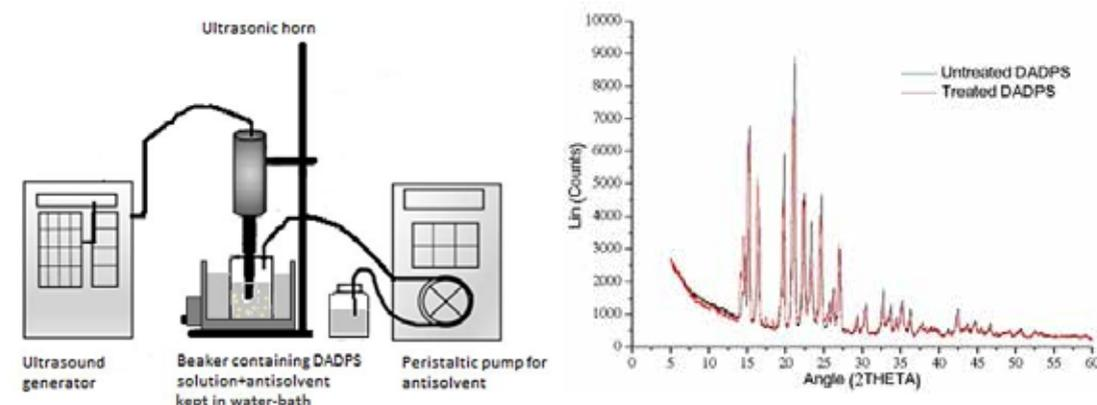
Figure 1: Schematic representation of ultrasonic treatment for size reduction of DADPS in antisolvent crystallization
