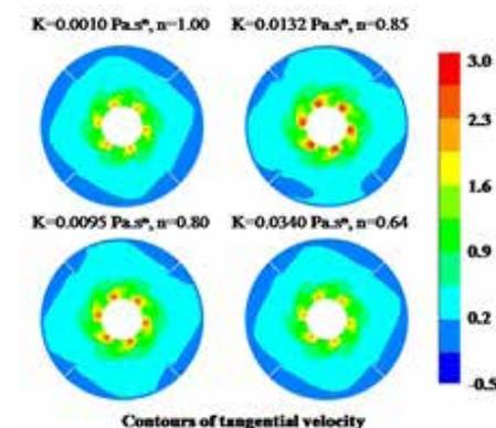
Fig 2. Contours plots of the tangential velocity plotted on the XZ plane (6-blade Rushton turbine)
