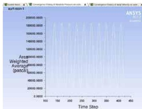
fig 3: Sinusoidal pressure variation profile graph
