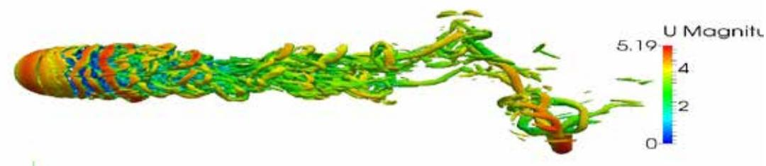
Figure: Velocity iso-contours for flow past a sphere obtained from fully resolved DNS implemented on a hexahedral mesh configuration of 128 Million cells, using a second order accurate central differencing scheme.
