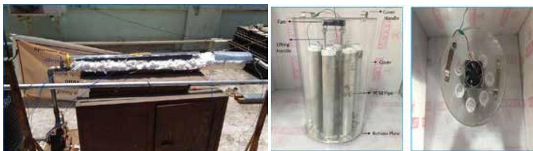
Figure 1: Thermal diode receiver experimentation under the sun.
