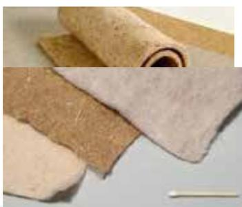
**Fig.4 Composite made from natural fibre**
