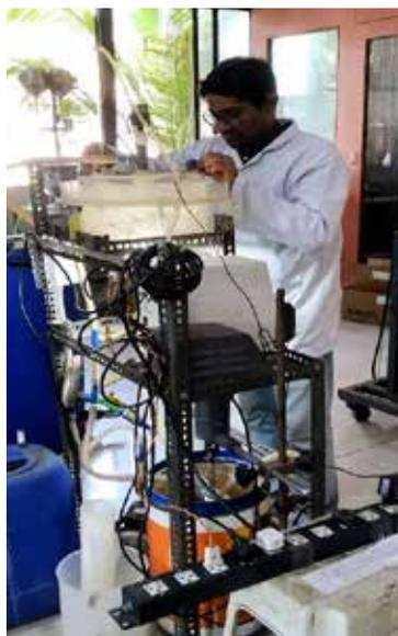
Pulsed Disk and Doughnut Extraction Column Setup
