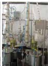
Closed-loop absorber-desorber setup for CO<sub>2</sub> capture
