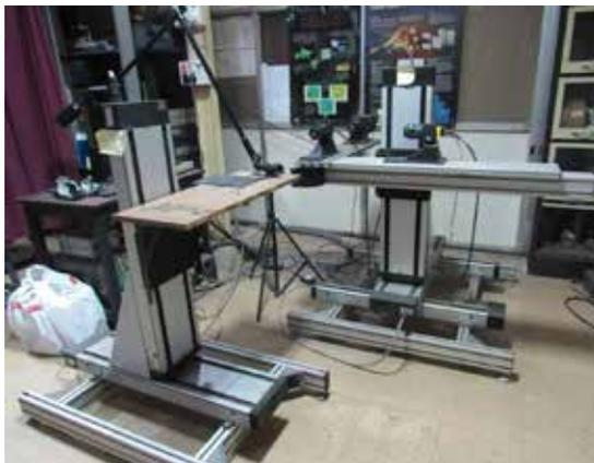
Particle Image Velocimetry Setup
