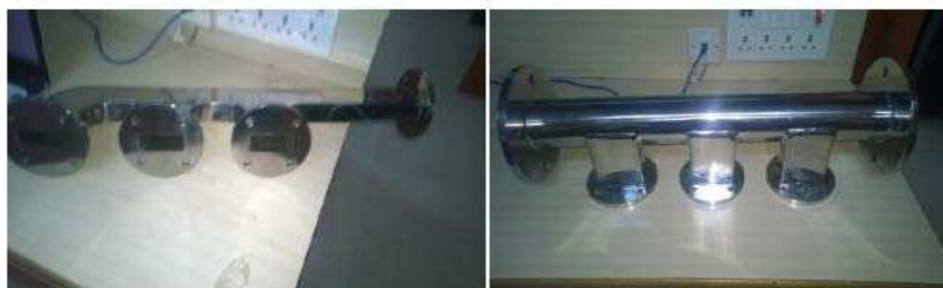
Fabricated waveguide and cavity of microwave reactor
