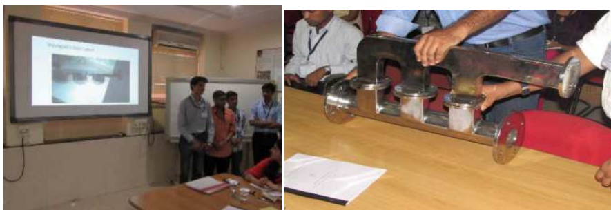
Fabricated waveguide and cavity of microwave reactor
