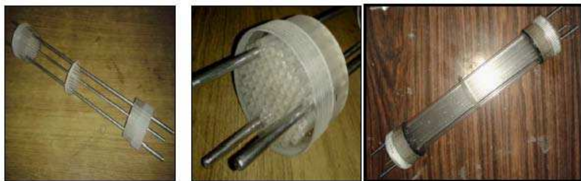
Module of the Reactor without Capillaries and A fabricated capillary module
